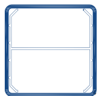
SECTION A-A LINE POST STIFFENER ALUMINUM INSERT
